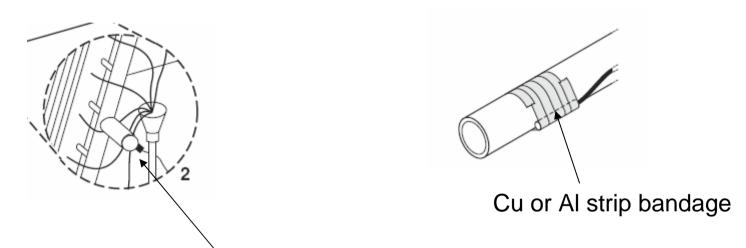
The sensor must be fitted on outlet (gas) refrigerant pipe
