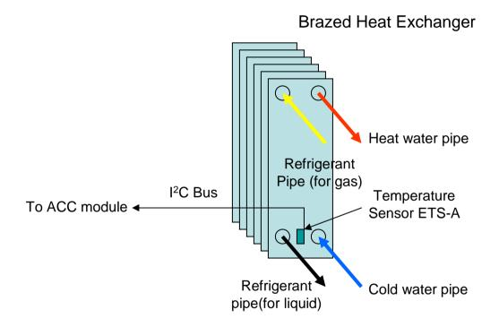
There must be proper temperature connection between heat exchanger and sensor. It must not be influenced by outdoor temperature.
