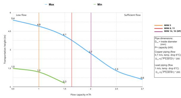
Parameters of hydraulic capacity of the indoor unit (unit with equipment)
