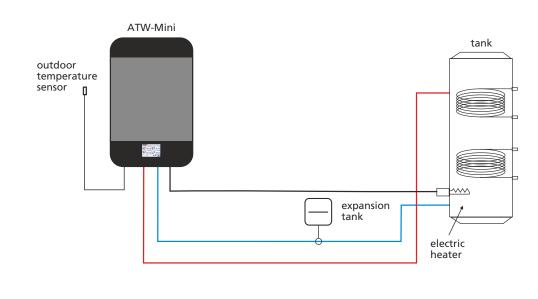
Example 3: Heating system with equitherm regulation and 3-way valve for HDW heating.
