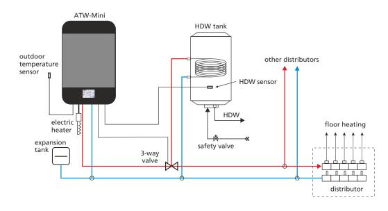
Example 2: Heating system with equitherm regulation and HDW pre-heating.
