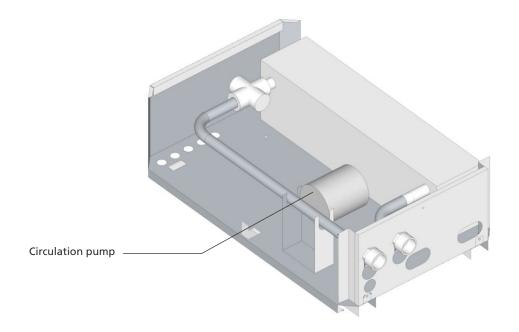
The indoor unit requires minimal maintenance. Use a wet cloth to clean the dust from the upper casing. Be extra careful when cleaning the heat pump during its operation. It is recommended to cleaning the indoor unit after the heating season and when it is disconnected.
